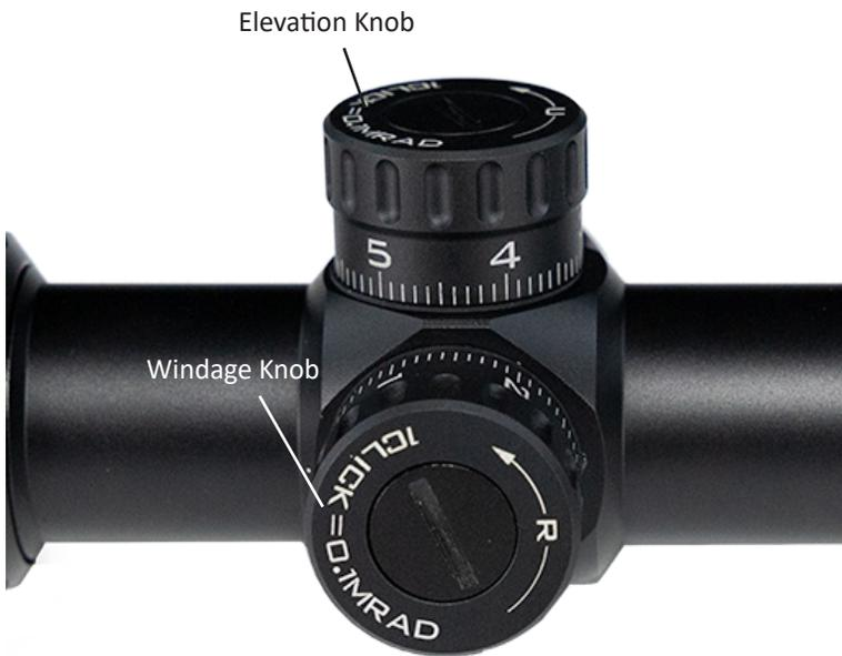
The TS-12X features 1/10 MIL or 1/4 MOA clicks on both the elevation and windage knobs. The click value specific to your optic is engraved on the knob. The elevation and windage knobs feature a directional arrow which indicates the direction your impact is moving when the knob is adjusted.
