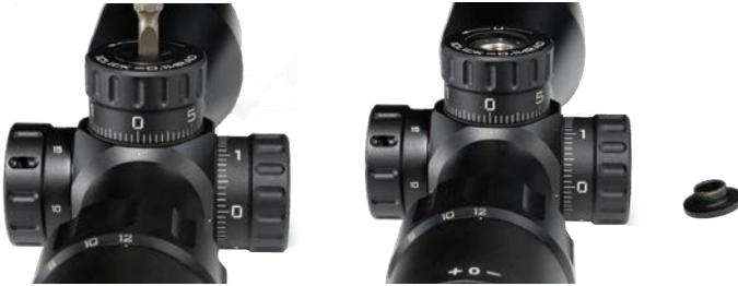
2. Completely lift the knob off and float it to read zero. When "0" is aligned, push down on the knob to place it in the locked position. Ensure that the knob is in fact free floating, by listening for audible clicks. You should NOT hear audible clicks while floating your knob.
