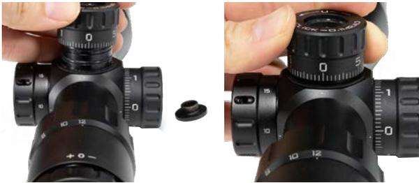
3. Once you've verified that your knob aligns to read "0" and is locked in place, re-insert the center screw and retighten it by turning the flathead screw driver clockwise.
