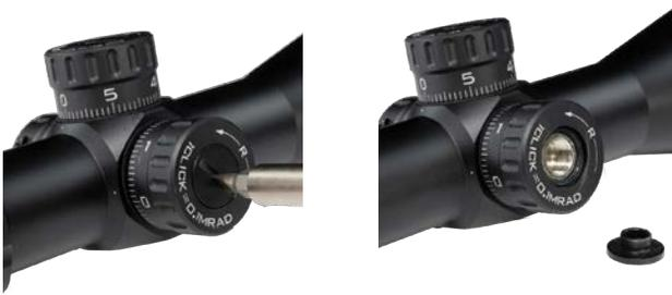
5. Completely lift the knob off and float it to read zero. When "0" is aligned, push down on the knob to place it in the locked position. Ensure that the knob is in fact free floating, by listening for audible clicks. You should NOT hear audible clicks while floating your knob.
