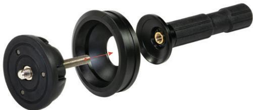
THE LEVELING HEAD IS UNASSEMBLED FOR COMPACT STORAGE. TO ASSEMBLE, INSERT THE SHAFT OF THE HALF-BALL MOUNT INTO THE CONVEX SIDE OF THE BOWL MOUNT. THREAD THE HANDLE ONTO THE HALF-BALL SHAFT.
