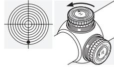
Turn the knurled knob of the elevation turret in the direction of H (counter-clockwise).
