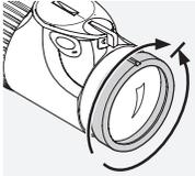
First turn the dioptic correction ring all the way to the left (counter-clockwise) and then to the right, until the reticle is optimally focused. The adjustment ranges depend on the individual
