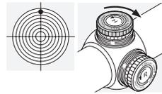
Turn the knurled knob of the elevation turret in the opposite direction to H (clockwise).
