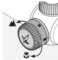
Using the parallax turret, you can adjust the optimum focus for every target distance thus preventing aiming errors due to parallax.
