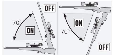
The rifle scope also switches off if the lateral tilt exceeds  $30^\circ$  (if you rest the weapon on your legs, for example).
