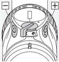
You can now adjust the brightness in the mode selected by means of the +/- button. To quickly find the optimum brightness, the button can remain pressed (sustained pulse). You can make fine adjustments by pressing the buttons once (individual pulse).
