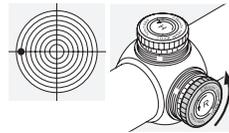
Turn the knurled knob of the windage turret in the direction of R (counter-clockwise).
