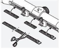
The cover provided serves to protect the exposed rail parts. It may be cut to the required size and pressed into the rail by hand.
