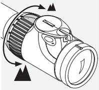
You can set the desired magnification by turning the (stepless) magnification adjustment ring through 180°. The scale on the adjustment ring allows simple and easy reading of the
