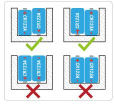
Install battery compartment and press it until it clicks - make sure the cover is closed on both sides. Open Close
