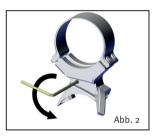
2. Loosen the grub screw with a hex key wrench 1,5mm.
