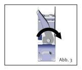
3. Open the clamping piece by turning the lever clockwise.
