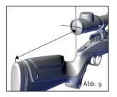
14. Bevor you tighten the screws, check that the optik is in the right position on the MONO-BLOC. The eye relief has to be adjusted according to the manufacturer's instructions and the reticle has to be aligned.
