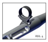
4. Position the mount on the receiver of the MONOBLOC.
