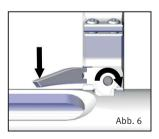
Fix the mount by tightening the threaded spindle with an external star wrench TX8 with 1 Nm. Push the lever downwards during tightening the threaded spindle so that the clamping piece stays closed.
