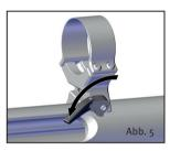
Swing the lever counter clockwise, to fix the mount with the clamping piece on the receiver of the MONOBLOC
