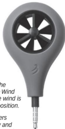
Note - The WeatherFlow WindMETER is included with the KILO2400ABS. For some smartphones, the WindMETER will not function properly due to incompatibilities from smartphone to smartphone. This is caused by insufficient drive current through the audio jack. Some newer smartphones no longer have an audio jack.
