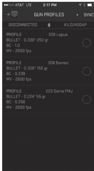
5. Now that you have one or more profiles created, you need to select which profiles are to be downloaded to your rangefinder. Press the grey circle next to the profile to select up to 4 profiles for synchronizing with your rangefinder. In this example 2 out of 3 profiles are set for synchronization:
