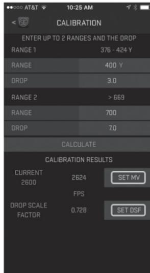
*After inputting the actual drop data as a function of known ranges, press CALCULATE and then press SET MV and SET DSF to apply your new MV and DROP SCALE FACTOR for better accuracy.*
