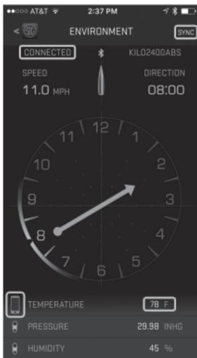
*After adjusting for wind direction and any environmental parameters, and verifying that the rangefinder is connected, press the SYNC button to update the rangefinder. You are now ready to range.*
