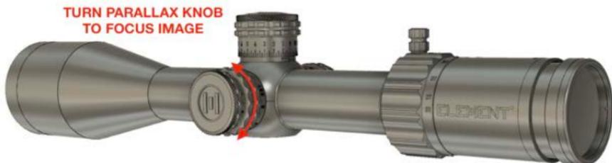
**Tip:** Place your rifle scope in a fixed position and change the position of your eye (up/down, left/right) while adjusting parallax. If parallax is not set correctly, there will be apparent movement of the reticle in relation to the target. Adjust the parallax until this movement is eliminated.
