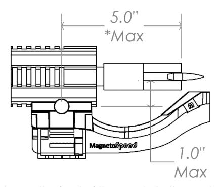
\* From the front of the muzzle to the center of first available rail slot
