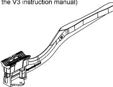
2. Insert plastic V-block adapter and screws. Note the raised ledge can go to the front or rear of the V-block. For Glocks and most rails with a single groove the ledge will need to be positioned forward in the V-block. For full rails with multiple slots the ledge works best towards the rear of the V-block.
