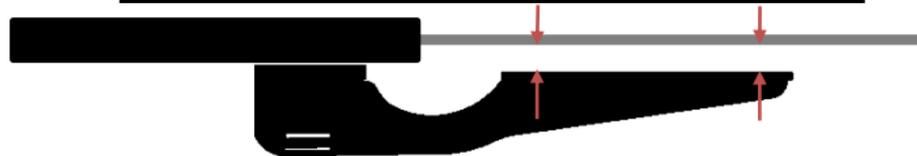
Use a cleaning rod to check the spacing of sensor 1 and sensor 2 from bottom bullet edge. Distances should be between 1/8" and 0.375" and they should be within 1/16" of each other.
