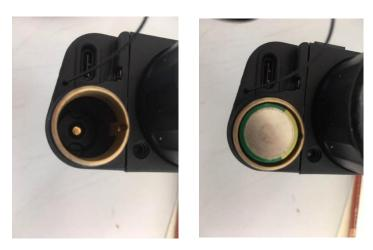
Fig. 5-1 Schematic diagram of battery installation
