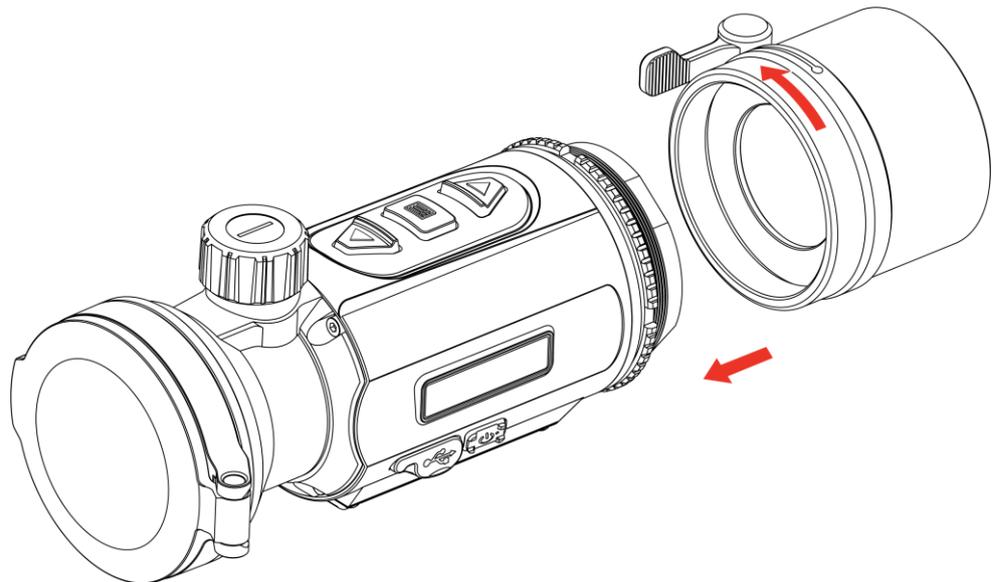
Figure 2-6 Install Adapter
