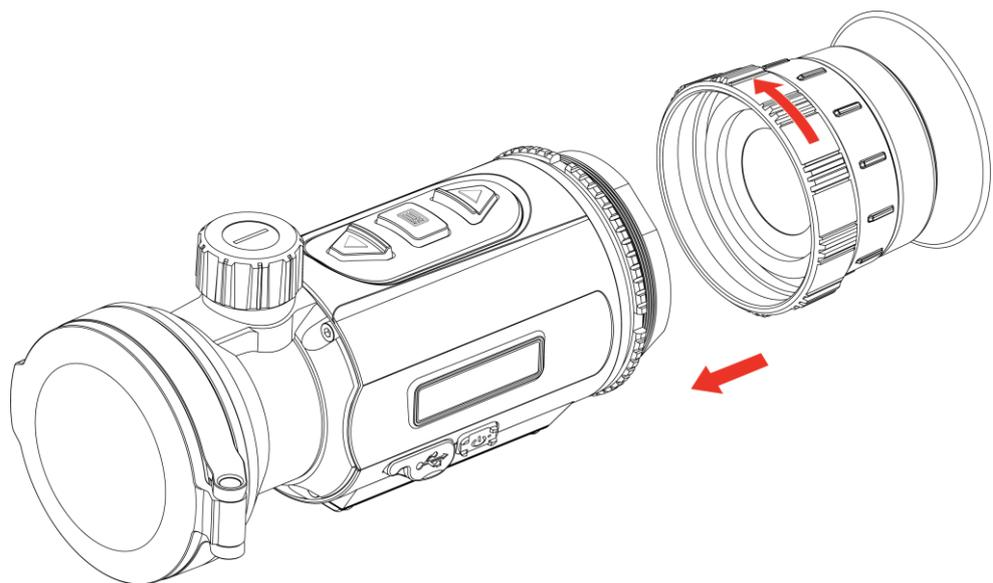
Figure 2-5 Install Eyepiece
