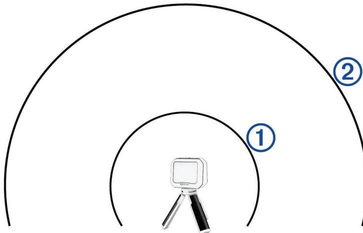
**NOTE:** The weapon can be positioned at any point around the chronograph as long as the weapon and chronograph are positioned 15 to 35 cm (5 to 15 in.) away from each other. You should choose a location that works best for your weapon.
