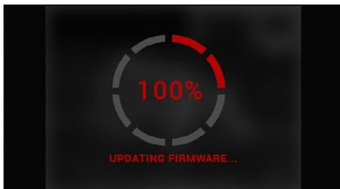
10. Please delete the Firmware file off of the microSD card after the process is complete. Or the system will try to update the Firmware every time you turn the monocular on.
