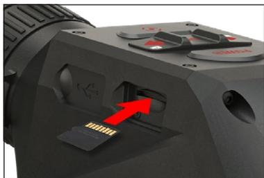
3. Use a thin object (small coin, paper clip) to lock the microSD card in place after inserting it into the slot.
