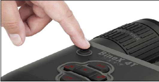
To TURN ON the device, press and hold the POWER button until you see the ATN splash screen.
