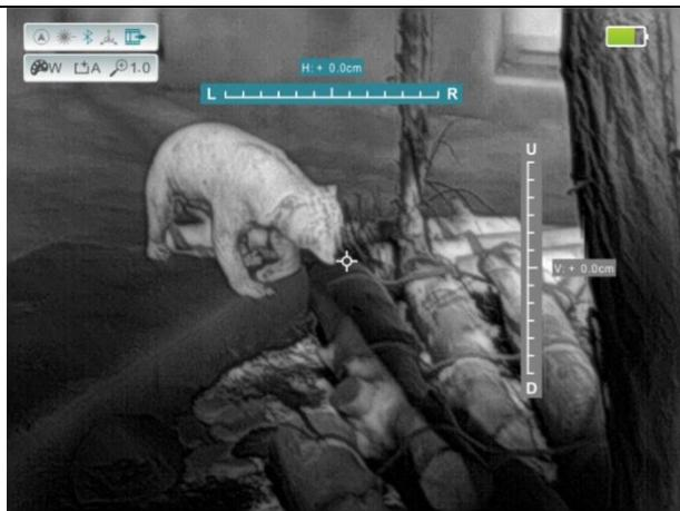
Figure 5-6. Reticle calibration interface
